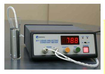
With the new Model 871 the measurement of dielectric constants has been very easy. Insert the probe in the liquid to been measured, adjust the two controls on the front panel and read the dielectric constant from the display. The Model 871 can accurately measure in low and high dielectric solvents, including mixtures.
